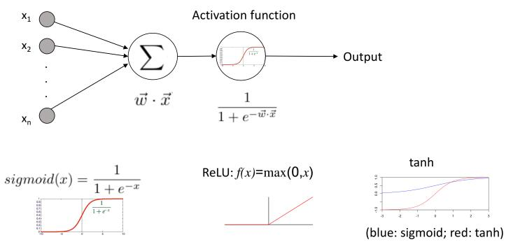
ReLU (Rectified linear function): typically applied for solving regression problems Sigmoid (logistic function): for classification Tanh: rescaled logistic sigmoid function
