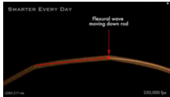
Figure 5: High speed video of flexural wave
